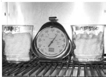
Both Core-Fill 500 and Core Foam Masonry Foam Insulation Turn Into Charred Masses in 54 Minutes at 400°F
