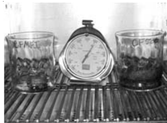
Both Core-Fill 500 and Core Foam Masonry Foam Insulation Turn Into Charred Masses in 54 Minutes at 400°F
